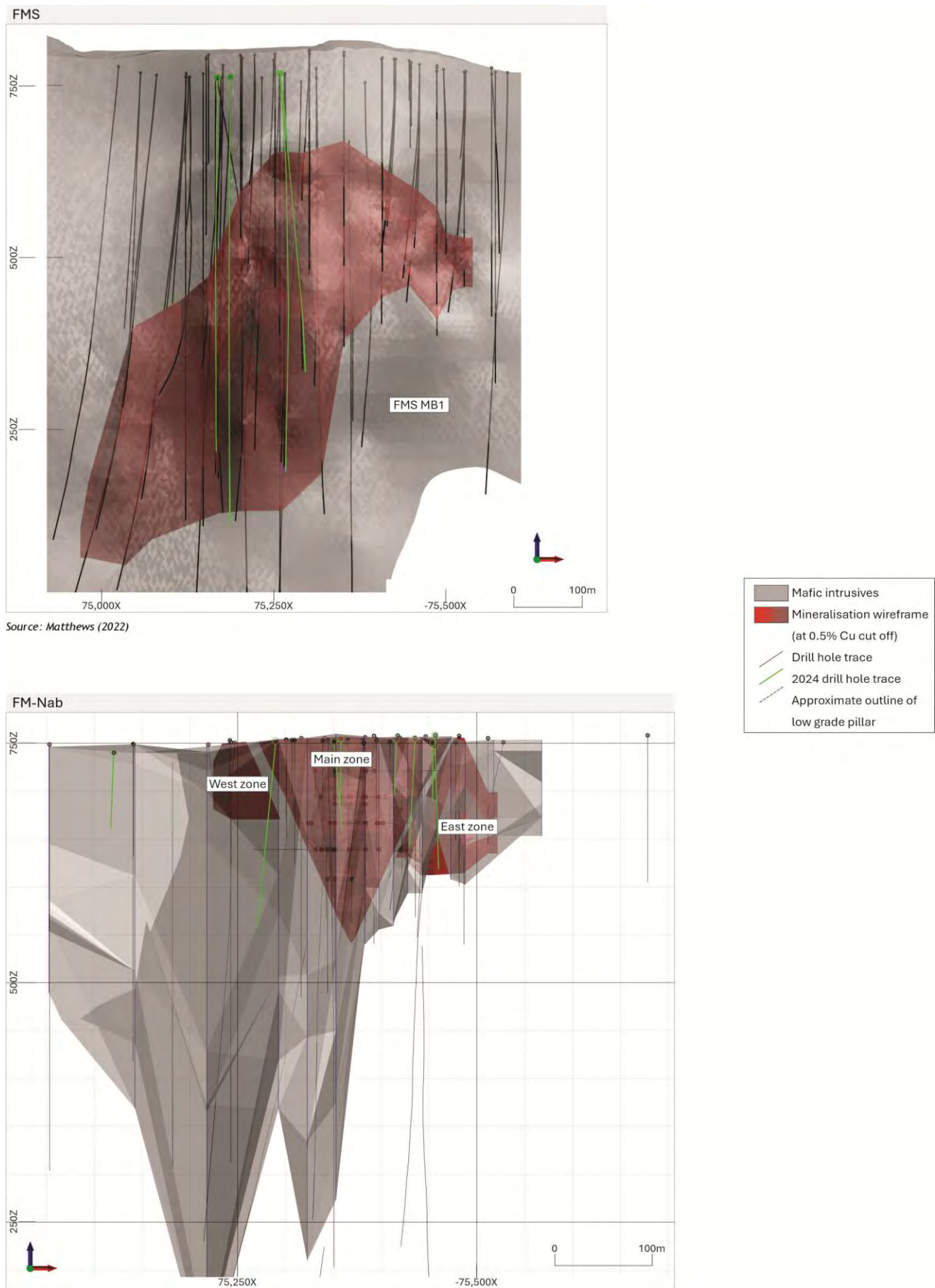
Figure 9: FMS and FM-Nab - Mineralised domains in relation to mafic intrusives and drill hole traces.
