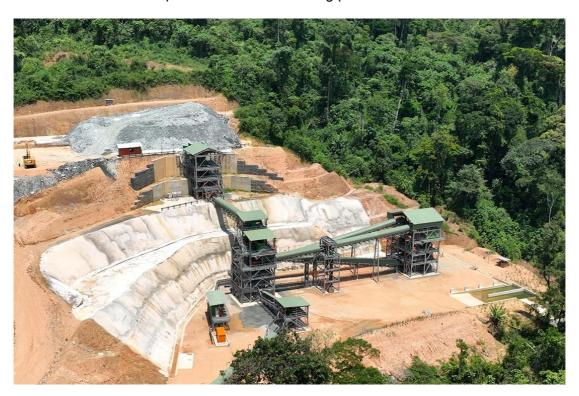
2. Crushing plant and crushed ore stockpile
