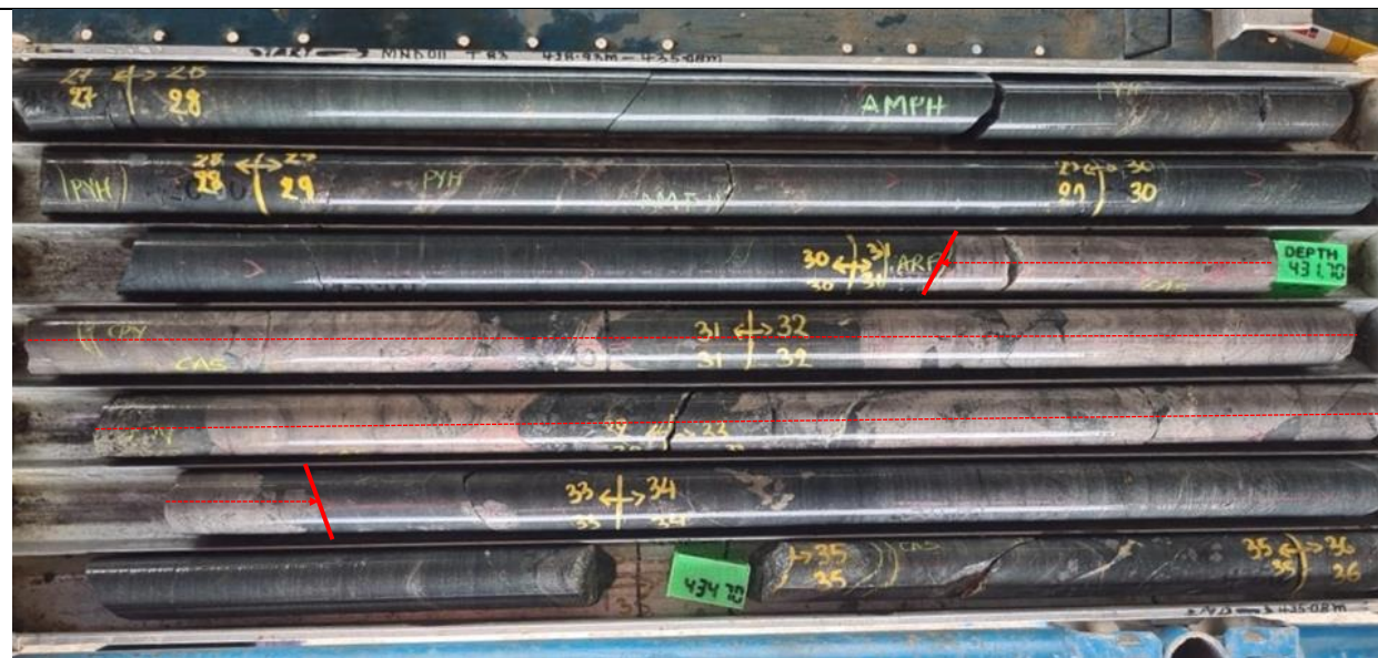
Figure 1: Highly mineralised cassiterite (pink) in Hole MND011 at Mpama North, including a zone of massive cassiterite veins (annotated with red dashed lines)
