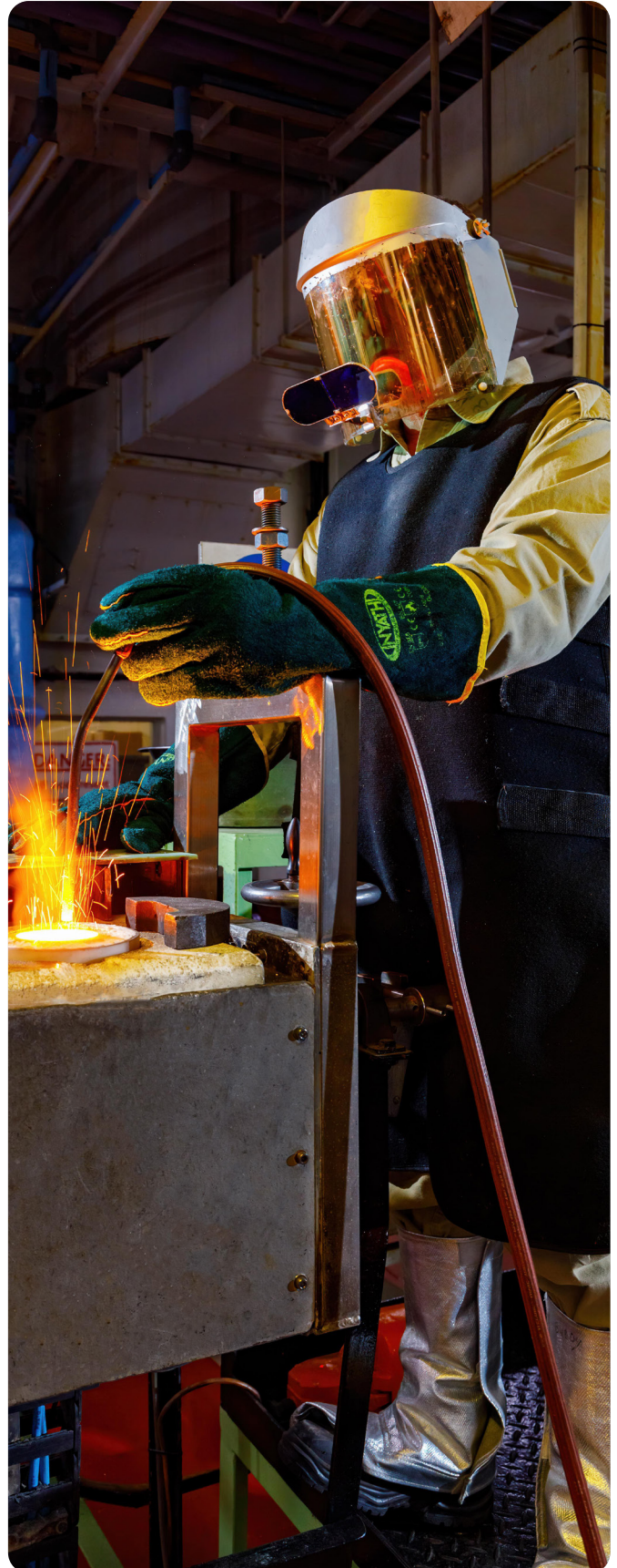
Casting of palladium ingots at PMR
