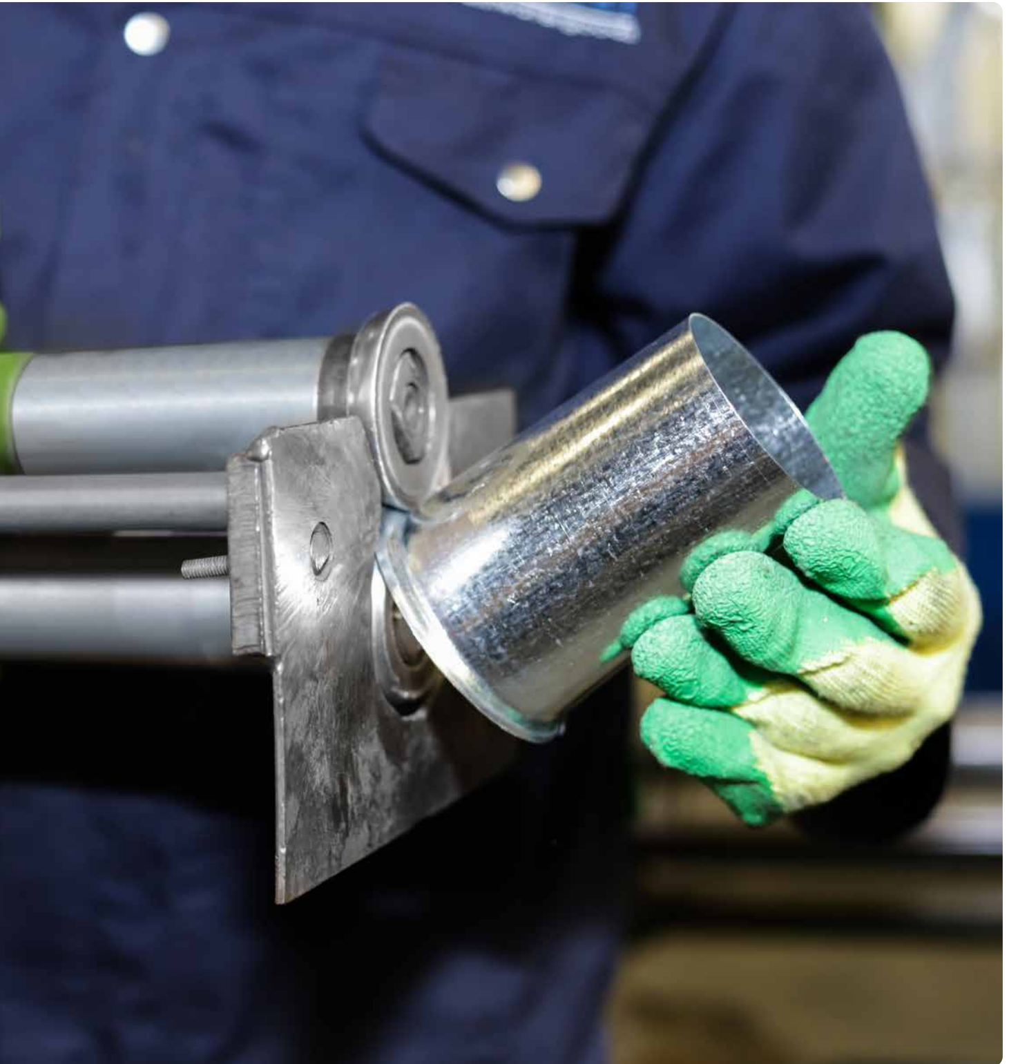
Premier Rainwatergoods: Flanging of round outlet.
