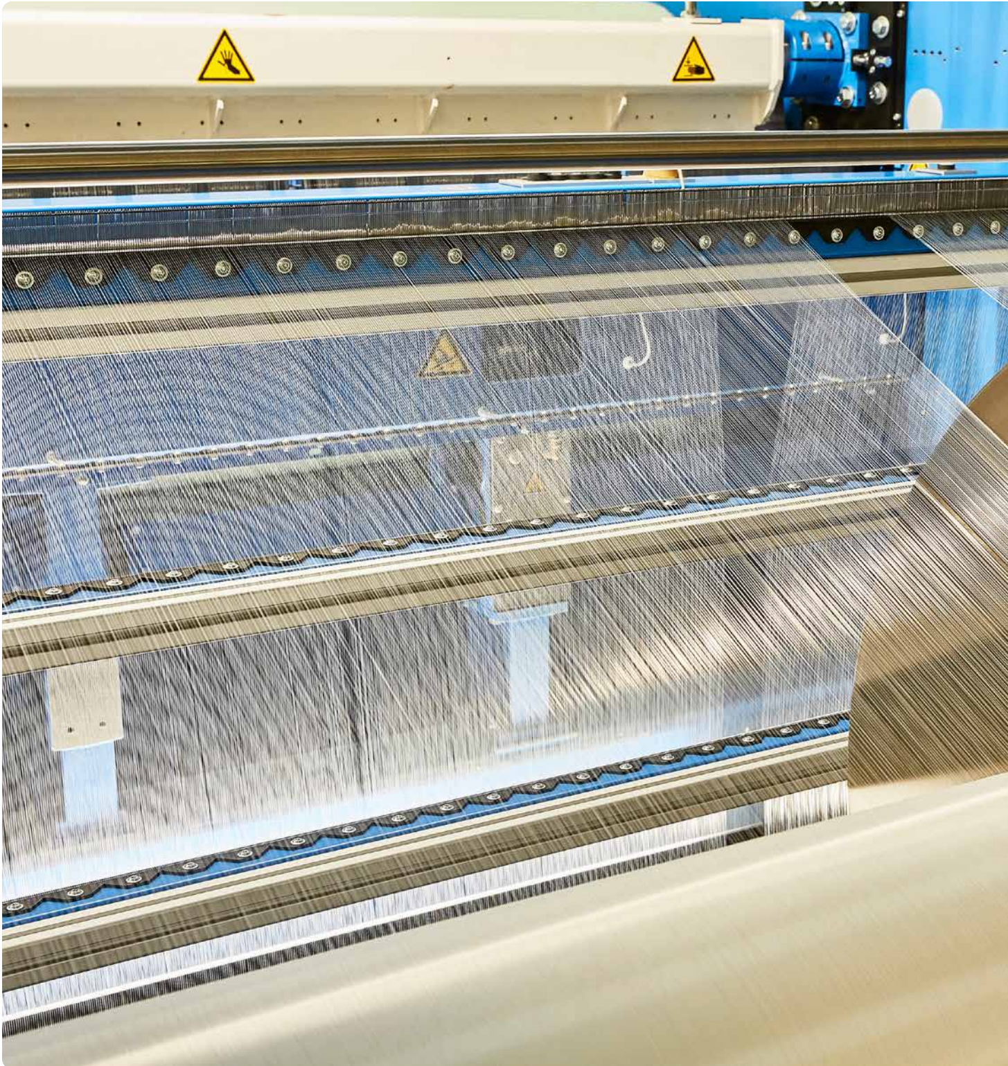
Romatex: The Maliwatt process of stitchbonding.
