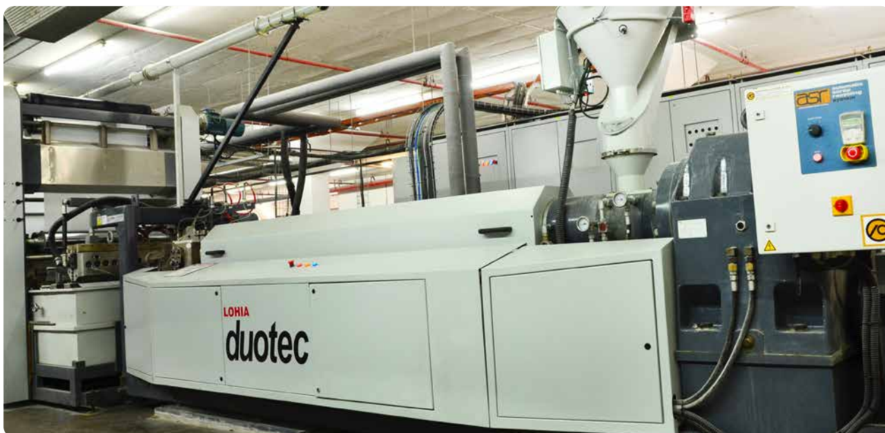
Integrated Polypropylene Products: New extruder machine that extrudes raw polymer materials into tape.
