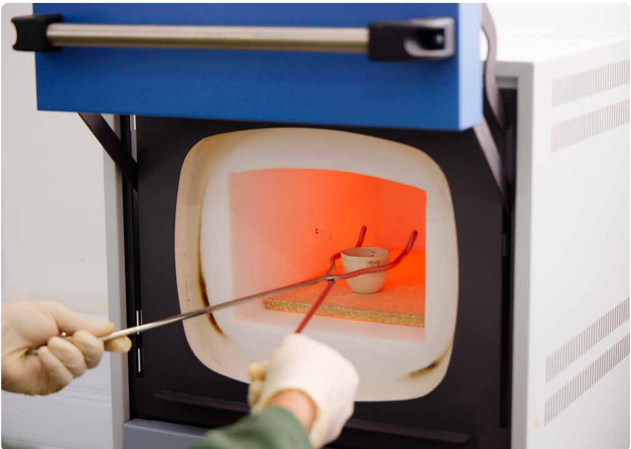
Gold Reef Speciality Chemicals: Solids content testing in furnace.
