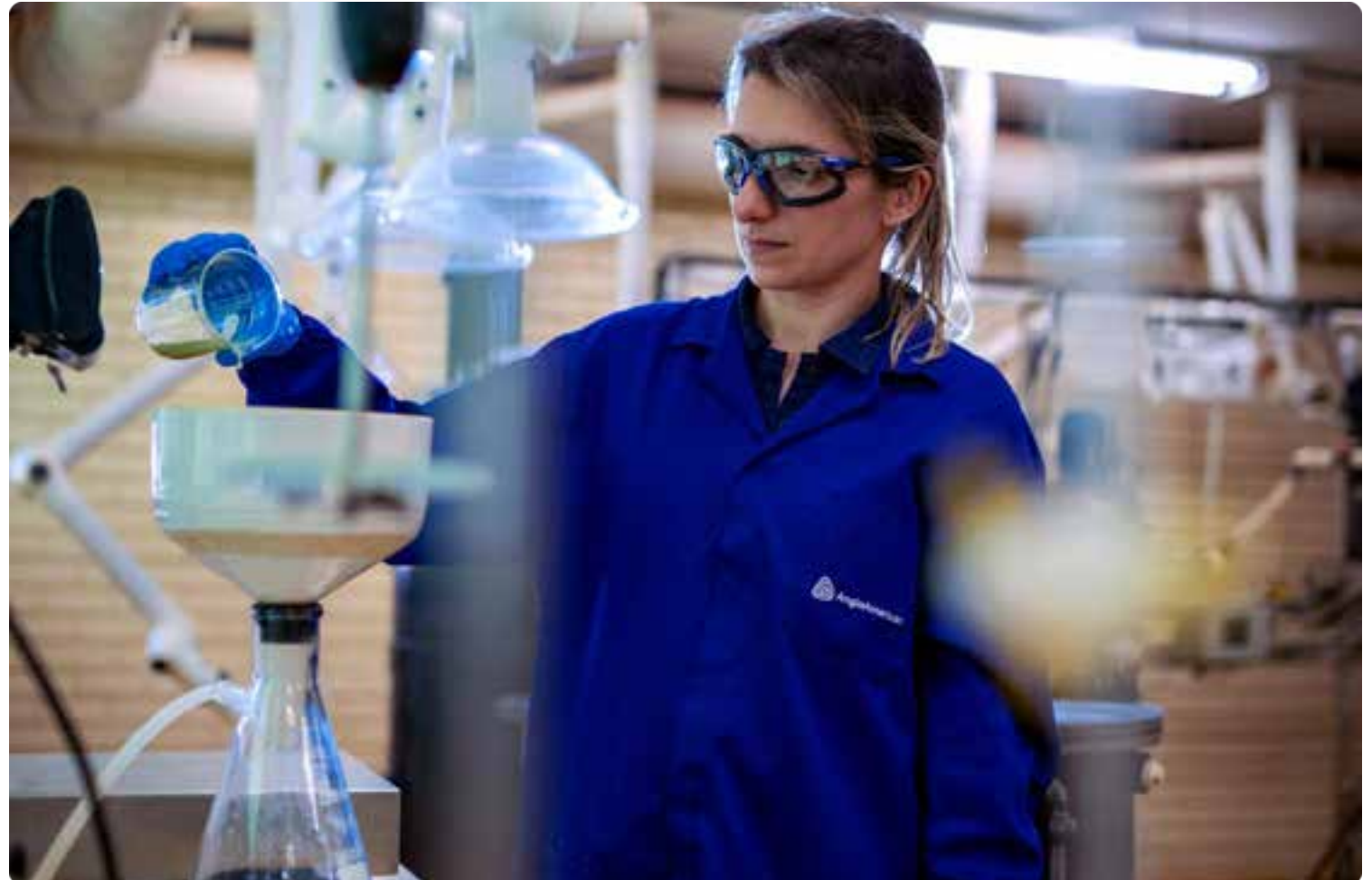
Process engineer Naiara Nascimento working with a pregnant leach solution enriched with soluble nickel, derived from comprehensive tests conducted in the leaching pilot plant at our Barro Alto operation in Brazil.
